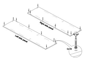
Fix the dowels in the holes of all the panels.
