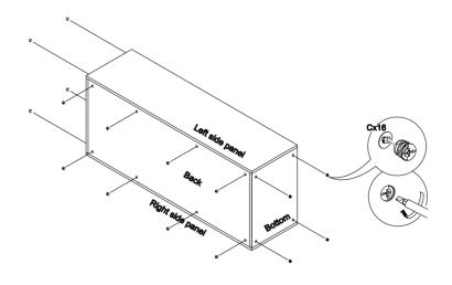
Fix the adjustable shelves. Use the hole plugs to cover the exposed holes.
