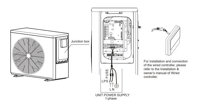
The ground fault circuit interrupter must be 1 high-speed type of 30mA(<0.1s). Stated values are maximum values (see electrical data for exact values). Leakage protection switch must be installed to the power supply of the unit. Equipment must be grounded.
