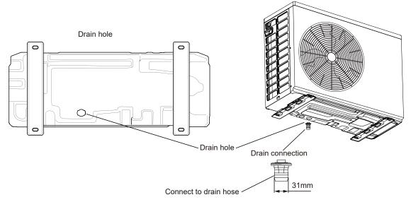
For collecting the condensed water and discharging it centrally, please connect the unit's drain hole to drain hose (30mm) by using the Drain Connection which included in the accessory.
